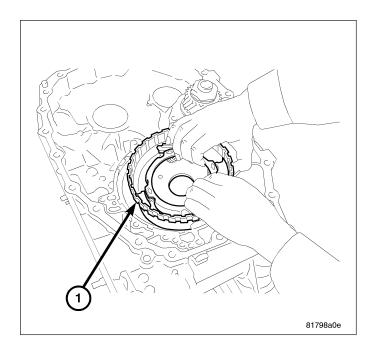
55. Remove the needle bearing (1) from the planetary carrier.
