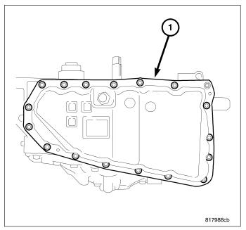
39. Remove the oil pan gasket (1) from the transaxle case.
