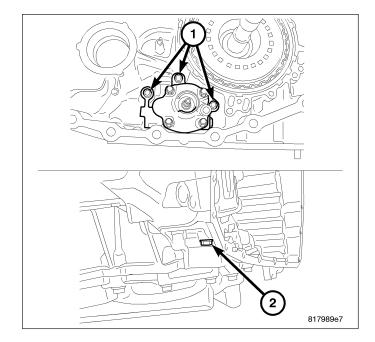
NOTE: One of the oil pump retaining bolts is installed from the outside of the transaxle case into the rear part of the oil pump.
