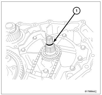
22. Remove the adjusting shim (1) from the drive sprocket, if necessary.
