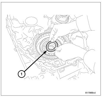
52. Remove the sun gear (1) from the planetary carrier.
