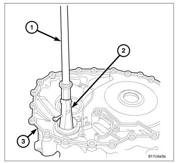
18. Remove differential side oil seal (1) from converter housing using a screwdriver. (2WD)
