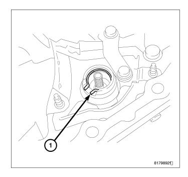
28. Remove the reduction gear assembly (1) from the transaxle case.
