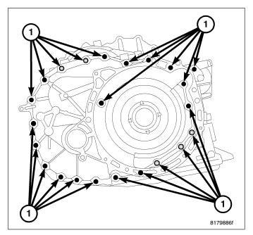
16. Remove the converter housing (1) by tapping with plastic hammer.
