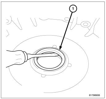
20. Remove outer race (1) of differential side bearing from converter housing using a suitable punch.
