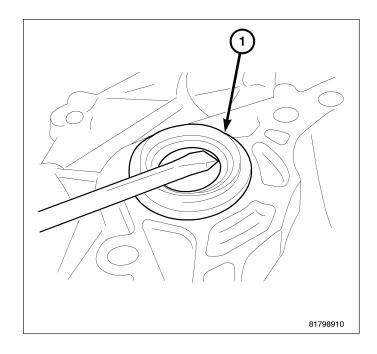
19. Remove converter housing oil seal (1) from converter housing using a screwdriver.
