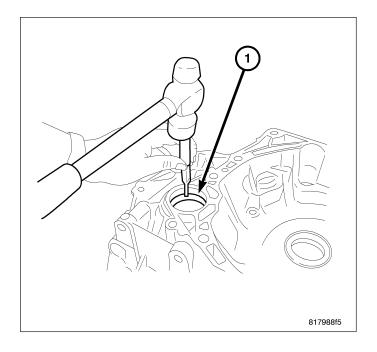
21. Remove and discard the O-ring (1) from the input shaft.
