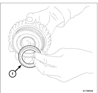
54. Remove the planetary carrier assembly (1) from the transaxle case.
