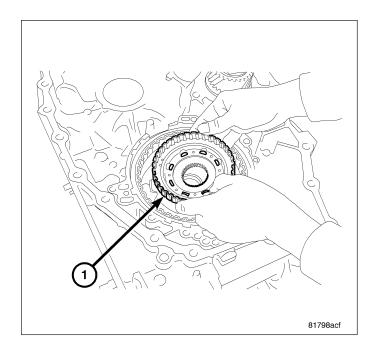
53. Remove the needle bearing (1) from the sun gear.
