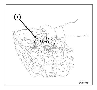
51. Remove needle bearing (1) from forward clutch drum side of the sun gear.
