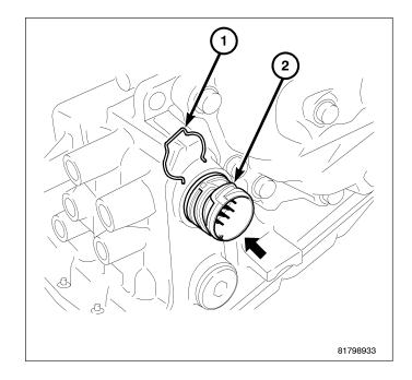
12. Remove CVT fluid cooler (1) from transaxle case. Remove and discard the CVT fluid cooler o-ring.
