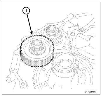
29. Remove the differential assembly (1) from the transaxle case.
