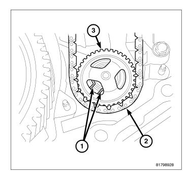
26. Remove the thrust washer (1) from the oil pump cover.
