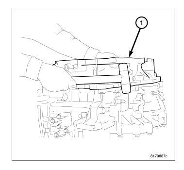
17. Remove outer race of reduction gear bearing (1) from the converter housing using Puller 7794-A and Slide Hammer C-637.
