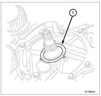
27. Remove the snap ring (1) from the oil pump.
