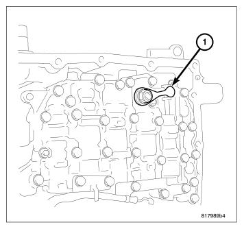
60. Use this picture when removing valve body attaching bolts.
