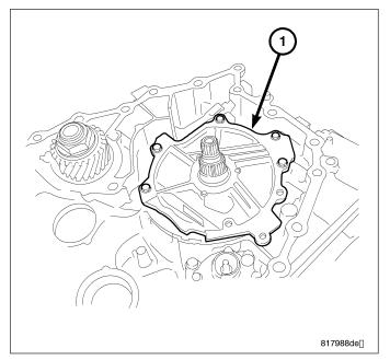
36. Remove and discard the seal rings (1) from the reaction shaft support.
