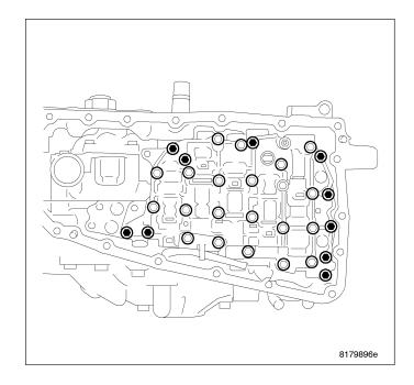
CAUTION: Tilt the valve body assembly away from the transaxle case on the manual shaft side to ease removal. Pay attention to completely remove the terminal body from the transaxle case.
