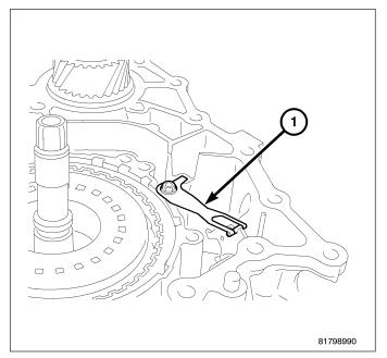
50. Remove the forward clutch assembly (1) from the transaxle case.
