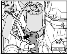
Remove rightly. . DA nagswayo V vahighvoo jha Remove right air duct hose, to do this lift retaining clips
