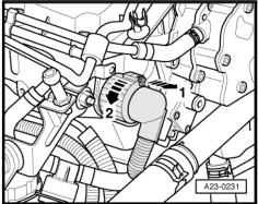
Disconnect connector -arrow- on fuel temperature sender -G81- and free wiring.
