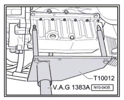
Insert engine support -T10012- in engine and gearbox jack -V.A.G 1383 A- .
