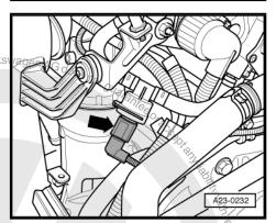
Remove coolant hose between engine and radiator -arrows-.
