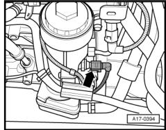
Disconnect connector -arrow- on engine speed sender -G28-using assembly tool -T10118- .
