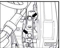
Loosen bolts -arrows- of assembly mounting on gearbox just a bit (less than 1 turn).
