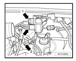
Pull vacuum hose -arrow- to brake servo off tandem pump.
