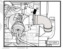
Remove connector -2- on radiator outlet coolant temperature sender G83- .
