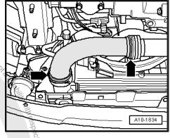
Unscrew nut -arrow- and take retainer for wiring harness off threaded stud.
