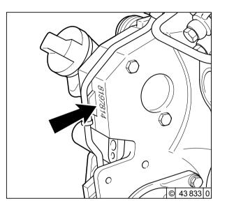
The engine number is stamped on the crankcase (arrow) and on the company plate.
