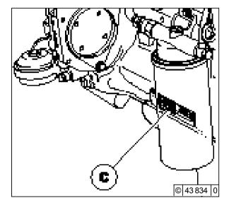
The company plate **C** is fixed to the cylinder head cover or the crankcase.
