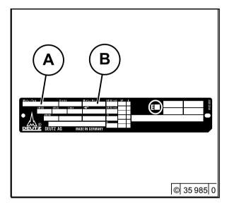
The engine type **A**, engine number **B** and the power data are stamped on the company plate. The engine type and number must be stated when purchasing spare parts.
