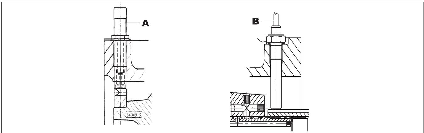
Fig. 1 - **A:** Flywheel pick-up coil
