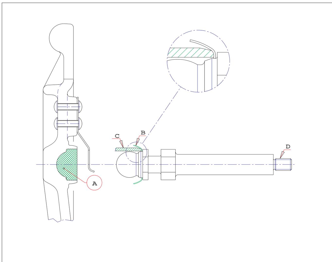
Fig. 7 - Fitting the clutch release fork.
