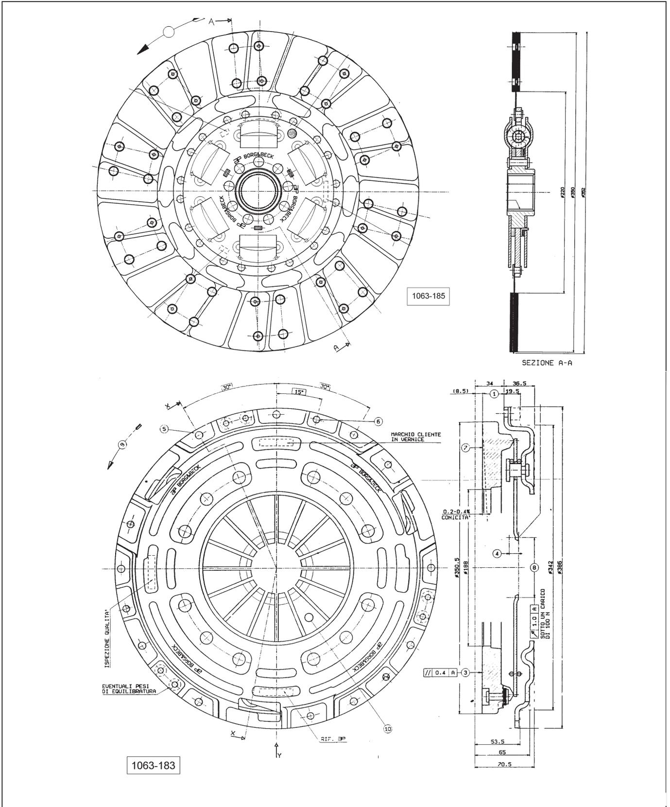
Fig. 5 - Clutch unit for **AGROPLUS 100**.
