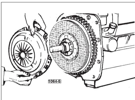
Fig. 9 - Installing clutch assembly through n. 5.9030.256.4/10 equipment.
