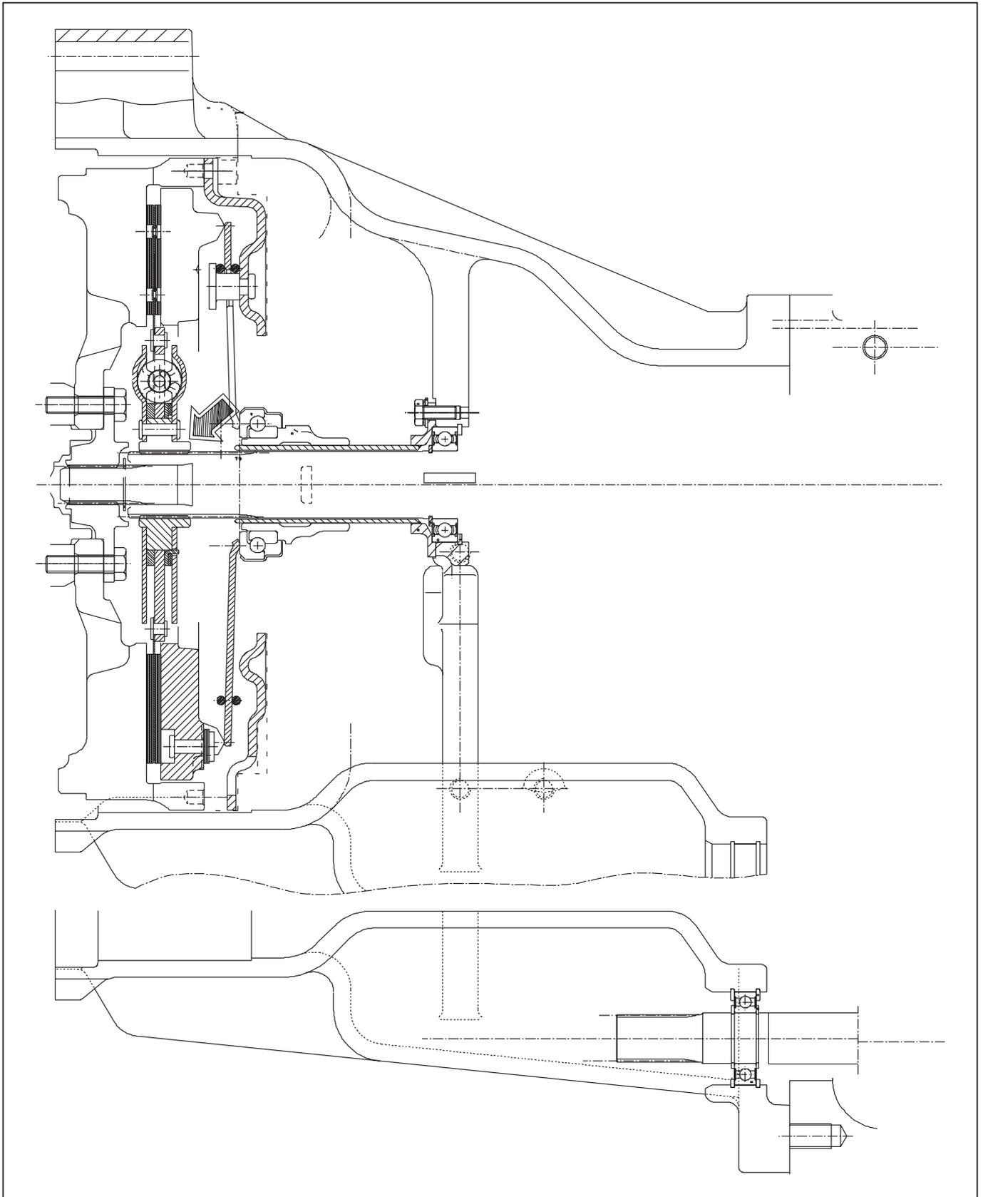
Fig. 3 - Clutch assembly.
