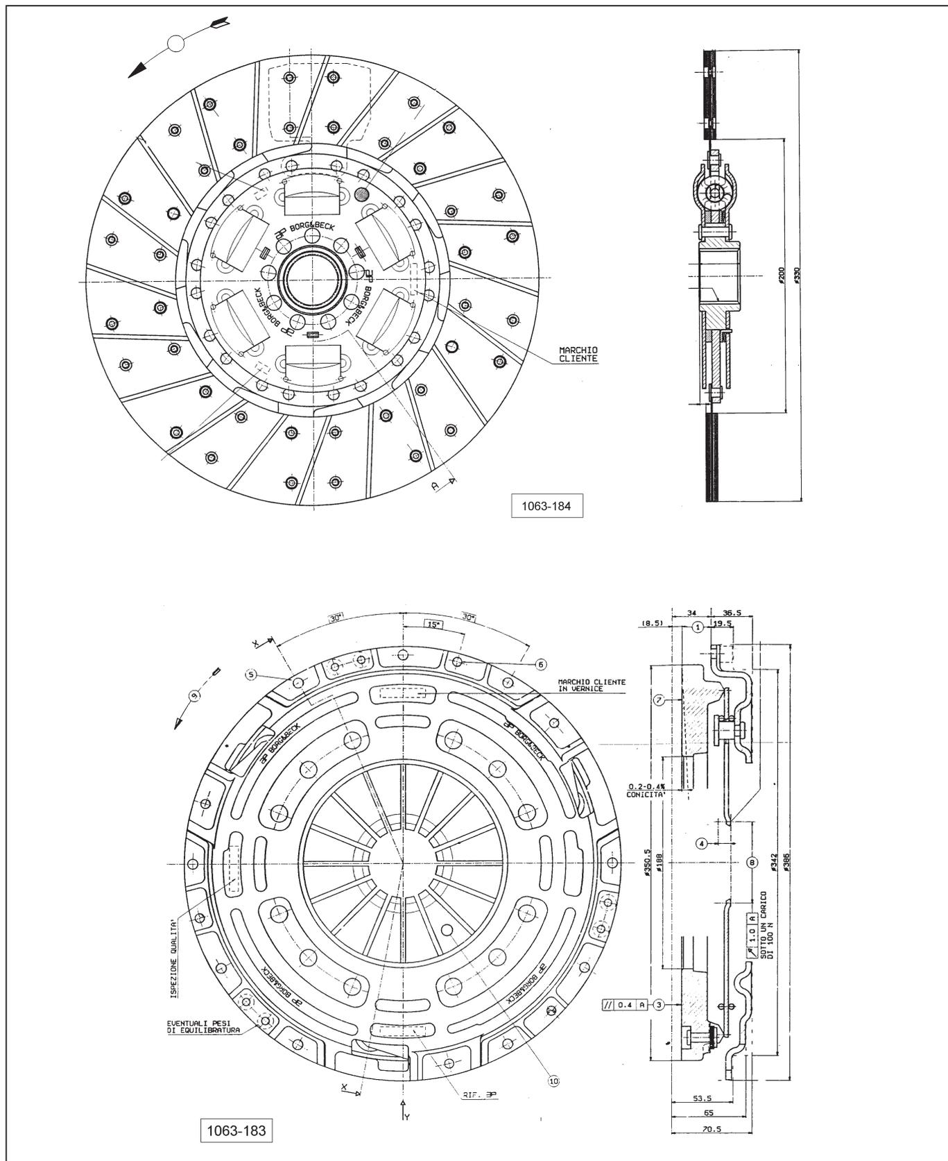
Fig. 4 - Clutch unit for **AGROPLUS 75-85-95**.
