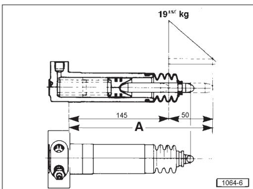
Fig. 10 - Clutch assembly hydraulic operating cylinder.
