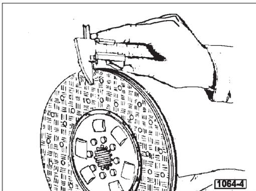
Fig. 8 - Checking clutch disk thickness.
