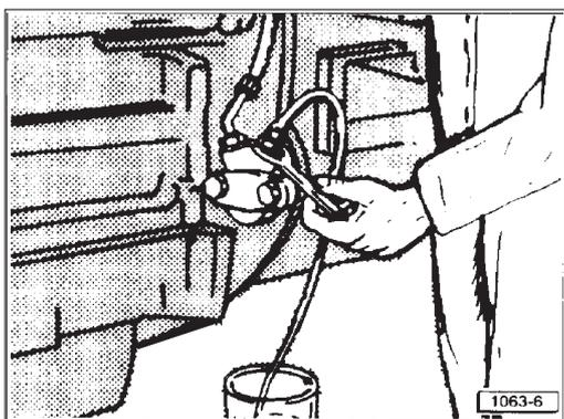
Fig. 11 - Bleeding the air from the clutch hydraulic circuit.
