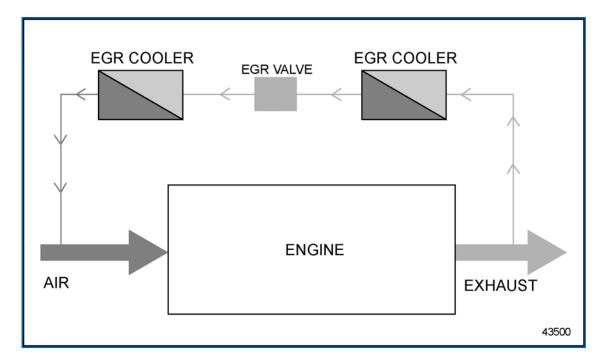
Air Flow Diagram Through Engine with EGR System
