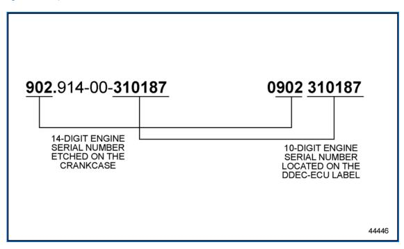
Engine Serial Number and DDEC-ECU Label
