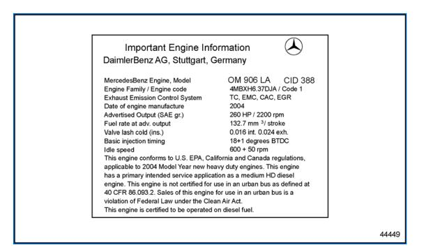
Emission Label for the 6-Cylinder EGR Engine
