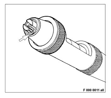
Use spindle to turn thread insert through snout until it is flush at front (arrow).
