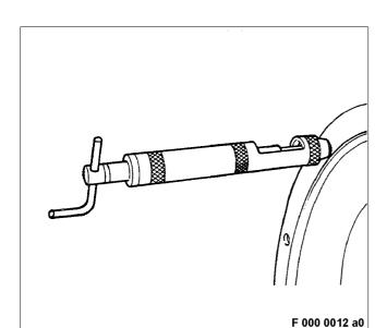
Mount installation tool on threaded hole and install thread insert without applying pressure to spindle.
