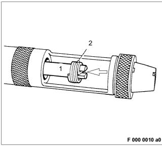
Insert thread insert (2) into spindle (1) in installation tool
