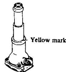
Fig. GI-13 Warning against over-stroke
