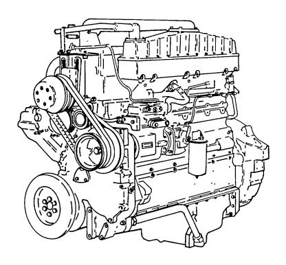
ENGINE, DIESEL, 6 CYLINDER INLINE, TURBOCHARGED, CUMMINS MODEL NTC-400 BC2 NSN 2815-01-156-6210
