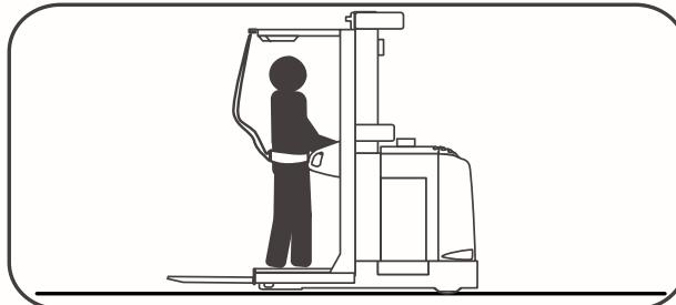
Operate truck from the position of the Operator.
