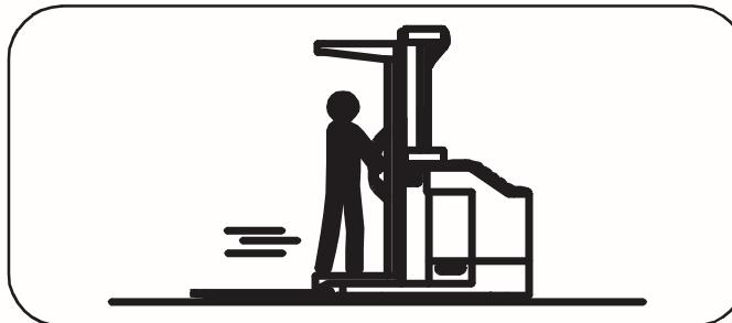
Before working on this truck, always turn the key switch to **OFF** and disconnect truck's battery connector (unless this manual states otherwise).
