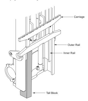
6. Hold the shorter block against the outer rail and lower the upright until inner rail rests on the block.
