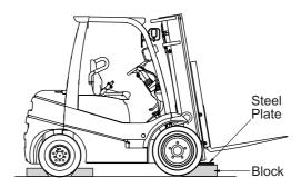
Tilt upright fully forward. This raises the drive wheels off the floor. Release the tilt control lever and turn engine OFF.
