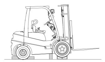
5. When maintenance work is completed, lower the truck to the floor by reversing the lifting procedure. Check to be sure no tools or equipment are under the truck or wheels.
