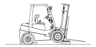
6. Insert blocking under the frame behind the drive wheels or slip wheel cradles under the drive wheels. If using blocking, check for safe clearance between drive wheels and floor and blocks.
