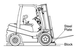
5. Tilt upright fully forward. This raises the drive wheels off the floor. Release the tilt control lever and turn engine OFF.
