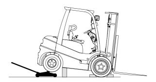
Put an equal amount of blocks under each side of the truck to provide a level working position.
