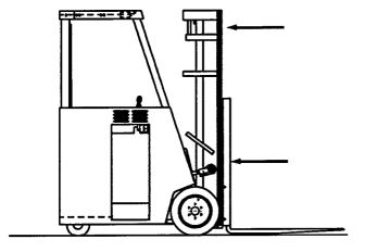
Check the overhead guard for damage. Be sure that it is properly positioned and all mounting fasteners are in place and tight and there is no structual damage.
