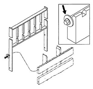
Check the load backrest for damage. Inspect the welds on the carriage and load backrest for cracks. Be sure that the mounting fasteners are all in place and tight.
