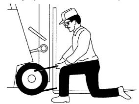
Check for the correct air pressure on trucks with pneumatic tires.
