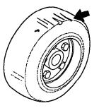
Check all wheel mounting bolts to be sure none are loose or missing.
