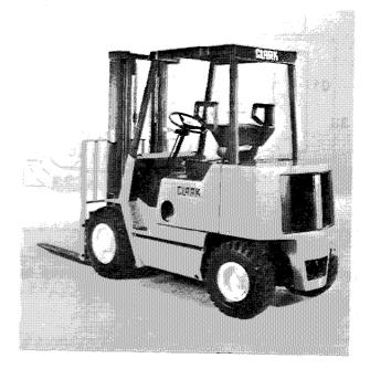
GPS MC, WC, and I models and GCS MC, WC, and I models are identified by the smooth hubcap at the center of the drive axle hub.
