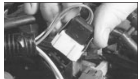
E Check all wiring block connectors are clean and secure.
