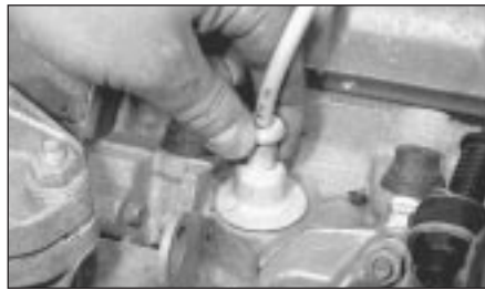
B Check that the HT lead connections at the spark plugs are clean and secure.
