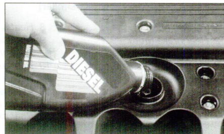
3.5 Topping-up the engine oil - Diesel engine shown
