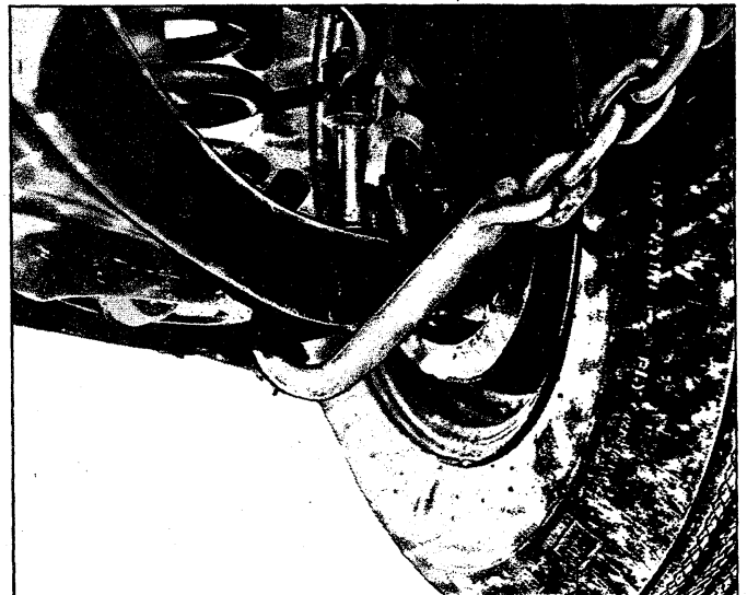
Fig. 23—Attachment of Towing Chain Hooks to Lower Control Arms
