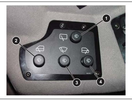
The "M" Series window wiper switches are on the top right of the cab. The switches are as follows:
