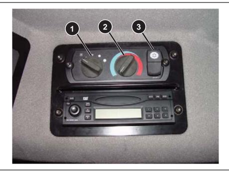
The "M" Series heating and air conditioning controls are now located on the top, right side of the cab. The controls are as follows:
