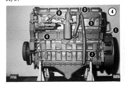
Visible on the left side of the engine are: the location for the magnetic pickup for an electronic tachometer (1), the access plug in the flywheel housing for locating top center for the No. 1 cylinder (2), the oil filler pipe (3), the accessory drive mounting (4), the crankcase oil gauge (dipstick) (5) and the governor (6).
