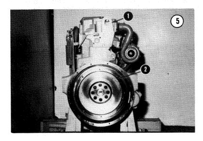
The rear view shows the rear lifting bracket (1) and the flywheel (2).
