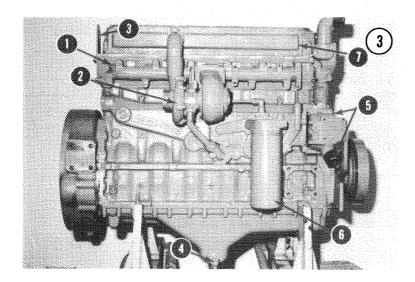
Located on the right side of the engine are: the exhaust manifold (1), the turbocharger (2), the rear lifting bracket (3), oil drain plug (4), the water pump and coolant inlet (5), the oil filter (6), the intake manifold (7), and the oil cooler (the oil filter is mounted to the oil cooler).
