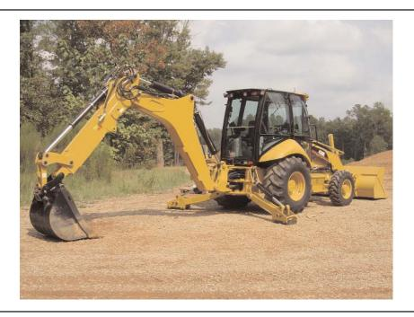
The new extendible stick (E-Stick) uses an external slider with a new wear pad design, which provides increased life and simplified serviceability. The E-Stick outer slider protects the inner slider from damage and debris and includes serrated gripping edges for improved clamping capabilities.
