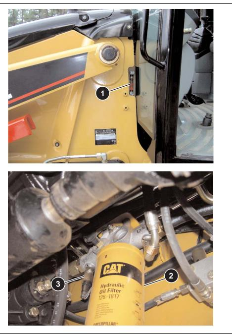
The hydraulic oil sight gauge (1) is located on the left side of the machine in front of the cab.
