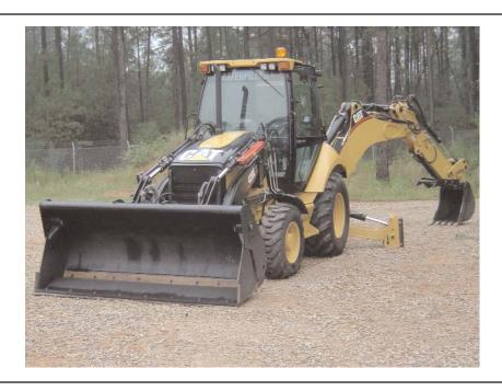
The new "E" Series cab with curved glass and contoured fenders gives the machine a distinct new look, improves serviceability, and provides superior visibility. The sleek hood is lowered for visibility and tilts forward for easy access.
