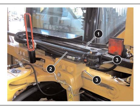
This illustration shows the optional powered sideshift (1) attachment. The powered sideshift moves the backhoe across the slider using a hydraulic cylinder (2). Wear pads (3) on the slider and powered sideshift assembly are serviceable.
