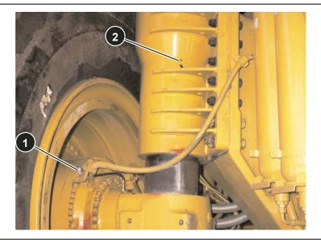
Check the front suspension cylinders for leaks or structural damage. Check the charge condition of the front suspension cylinders when the truck is empty and on level ground. Measure the charge height of the suspension cylinders and compare the dimension with the dimension that was recorded the last time the cylinders were charged. Recharge the cylinders with oil and nitrogen if necessary.
