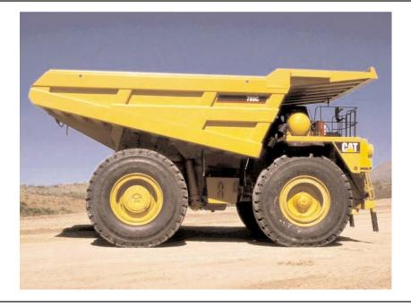
Shown is the right side of a 789C truck. The large air tank on the right platform supplies air for starting the truck and for the service and retarder brake system.
