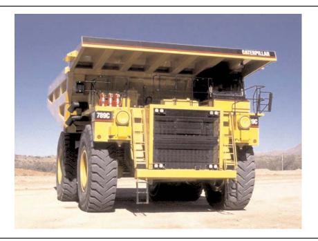
Shown is the front of a 789C truck. The 789C is similar in appearance to the 793C and may be difficult to identify from a distance. The 793C can be identified by the four air filters and the diagonal access ladder. The 789C has only two air filters and is equipped with two vertical ladders.
