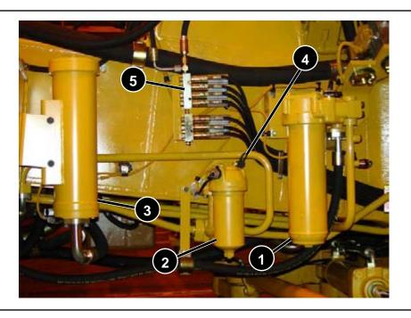
Located behind the right front tire is the transmission charging filter (1), the transmission lube filter (2), and the torque converter charging filter (3). Transmission oil samples can be taken at the Scheduled Oil Sampling ( $S \cdot O \cdot S$ ) tap (4).
