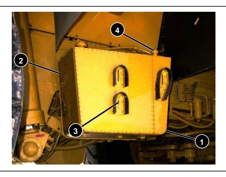
Shown are the transmission hydraulic tank (1) and the hoist, converter and brake hydraulic tank (2). Both tanks are equipped with oil level sight gauges.
