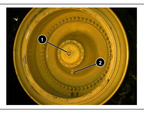
The front wheel bearing oil level is checked and filled by removing the plug (1) in the center of the wheel bearing cover. The oil should be level with the bottom of the plug hole. The fill plug is a magnetic plug. Inspect the fill plug weekly for metal particles. If any metal particles are found, remove the wheel cover and inspect the bearings for wear. The oil is drained by removing the drain plug (2).
