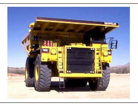
Shown is the front of a 789C truck. The 789C is similar in appearance to the 793C and may be difficult to identify from a distance. The 793C can be identified by the four air filters and the diagonal access ladder. The 789C has only two air filters and is equipped with two vertical ladders.
