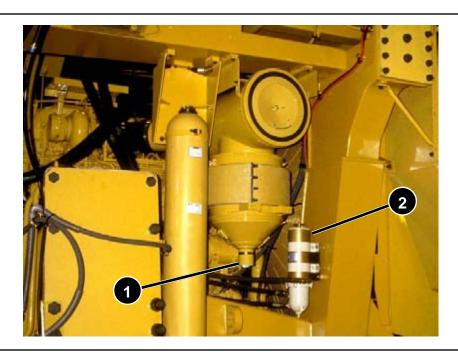
On the 785C truck, an air filter housing and a precleaner are located behind the front wheels on both sides of the truck. Check the dust valves (1) for plugging. If necessary, disconnect the clamp and open the cover for additional cleaning.
