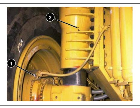
Check the front suspension cylinders for leaks or structural damage. Check the charge condition of the front suspension cylinders when the truck is empty and on level ground. Measure the charge height of the suspension cylinders and compare the dimension with the dimension that was recorded the last time the cylinders were charged. Recharge the cylinders with oil and nitrogen if necessary.
