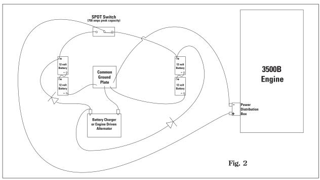
In the application of multiple engines, it is desirable to be able to operate any engine from any set of batteries or battery charger. The sketch below illustrates the use of redundant batteries. Notice the diodes are required in the application because the battery chargers/alternators are not dedicated to a specific set of batteries.
