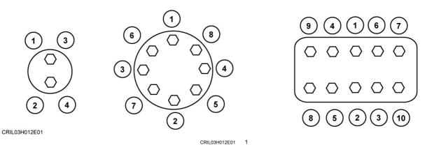
The numbers in the diagrams represent the order of tightening.
