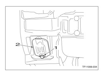
[2] Rotate the crankshaft one time in the reverse rotation direction to the 90° position before top dead center, then rotate in the correct direction to align the flywheel mark line (P/P) with the timing pointer. At this time, check that it is near No. 1 cylinder compression top dead center.
