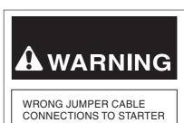
WRONG JUMPER CABLE CONNECTIONS TO STARTEF TERMINALS OR SHORTING ACROSS THE STARTER TERMINALS CAN CAUSE THE MACHINE TO MOVE SUDDENLY OUT OF CONTROL YOU CAN BE INJURED OR KILLED.
