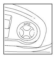
The adaptive seat control is located on the outboard side of each front seat. It is marked AUTO.
