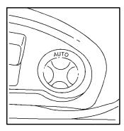
This control is located on the outboard sides of the front seats. With the ignition on, briefly press the top of the control where it is marked AUTO to activate the massaging lumbar feature.
