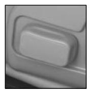
The power seat controls are located on the outboard sides of the front seat cushions.
