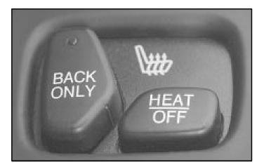
The buttons are located on the armrests. Press the buttons to turn the feature on. Press them again to turn off the heated seats. The feature will also shut off when the ignition is turned to OFF.
