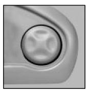
If your vehicle has this feature, the driver's and passenger's seatback lumbar support controls are located on the outboard sides of the seats.
