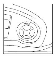
Push the top of the lumbar control located on the outboard side of the seat where it is marked AUTO briefly to activate the massage feature.
