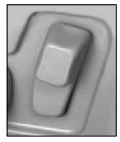
Press the recliner control located on the outboard side of the seat, forward or rearward to adjust the seatback.
