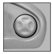
If you have this feature, the driver's and passenger's seatback lumbar support can be adjusted four ways by moving a single switch located on the outboard side of the seat.
