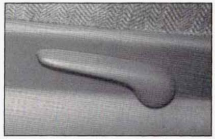
Lift the lever located on the outboard side of the seat to release the seatback, then move the seatback to where you want it. Release the lever to lock the seatback in place. Pull up on the lever without pushing on the seatback and the seatback will move forward.
