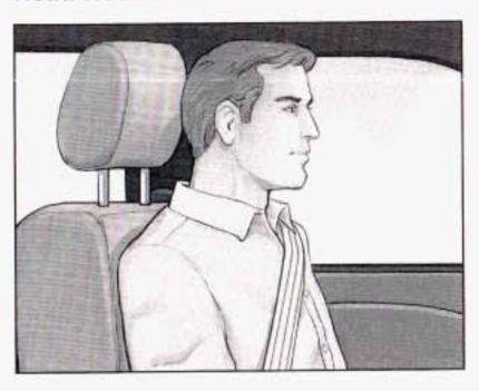
Adjust your head restraint so that the top of the restraint is closest to the top of your head. This position reduces the chance of a neck injury in a crash.
