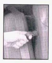
If your vehicle has this feature it allows you to have access to the trunk from inside of your vehicle. Pull forward on the seat tab, located on the front of the rear seat, to fold the rear seatback down.
