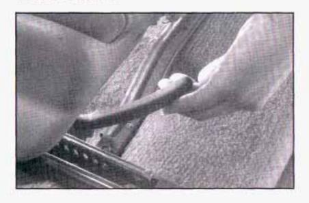
Lift the bar located under the front of the passenger's seat. This will unlock the seat. Slide the seat to where you want it and release the bar. Try to move the seat to be sure the seat is locked into place.
