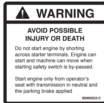
7. Jump starting - Located on the left side frame next to the starter.
