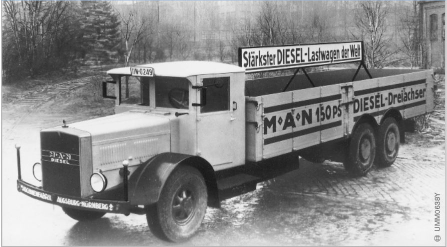
4 The most powerful diesel truck in the world from 1926 from MAN with 150bhp (110kW) for a payload of 10t
