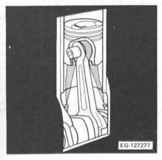
The lubrication system in the Turbocharged 400 series engines addresses the problem of on-the-spot immediate cooling with twelve oil cooling jets installed in the main bearing webs, two per cylinder. These cooling jets facilitate piston and wrist pin cooling, thus eliminating the possibility of heat build-up in these hardworking high friction areas.
