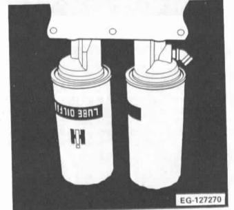
For ease of service all 300/400 series engines are equipped with two spin-on, throw-away type oil filters.
