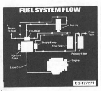
A fuel system which accurately meters the required amount of fuel for complete combustion, and provides complete governor control for power take off applications without the additional cost of add-on governors.
