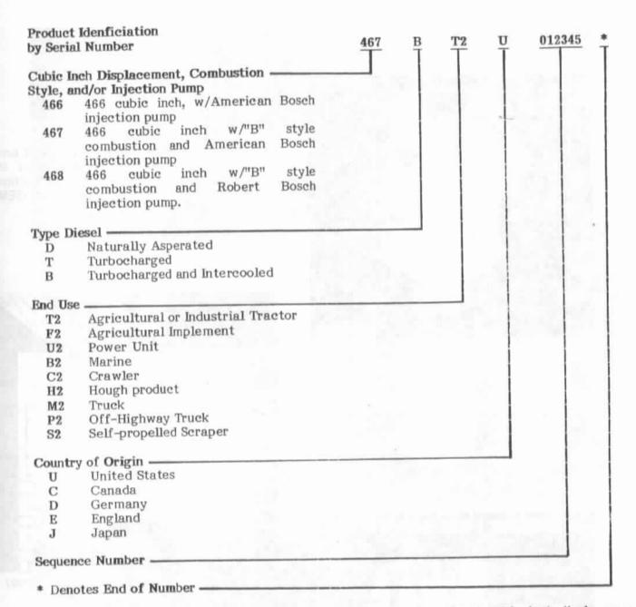
The engine serial number 467BT2U012345\* denotes an engine of 466 cubic inch displacement w/"B" style combustion, American Bosch injection pump, turbocharged and intercooled Diesel, for Agricultural or Industrial tractor, manufactured in the United States and identified as twelve thousand three hundred and forty five for production and record purposes.
