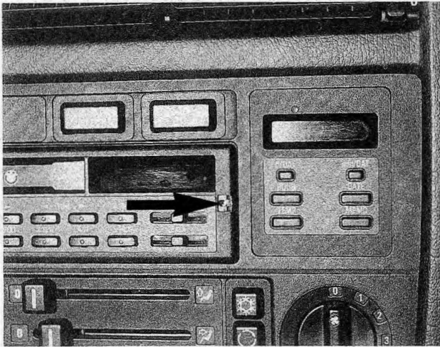
Fig. 4-13. Access hole (arrow) for internal-hex head screw used to retract retaining clip on late model BMW radios.
