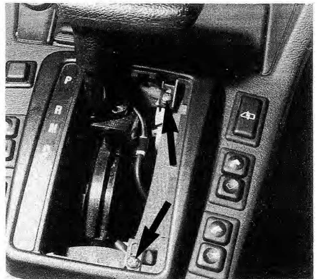
Fig. 4-6. Screws to be removed (arrows) for removal of shift lever trim panel.
