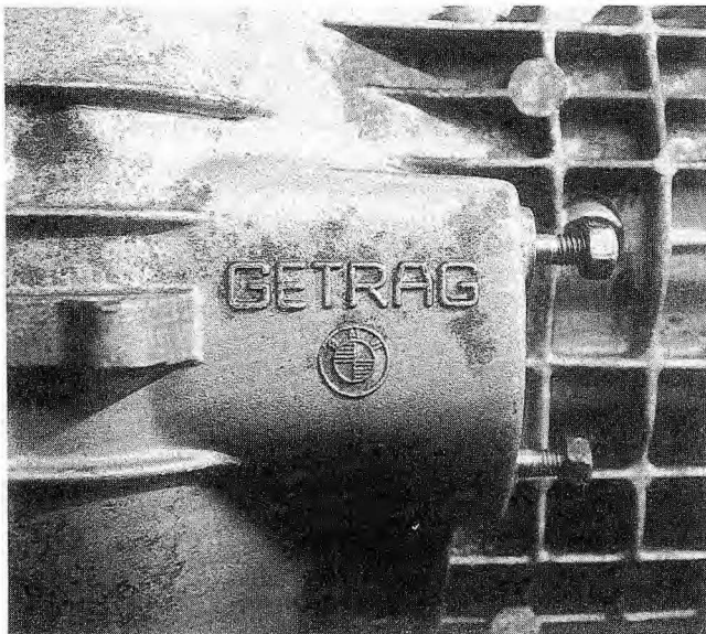
Fig. 1-3. Manufacturer's stamp for Getrag transmissions. ZF transmissions are similar.
