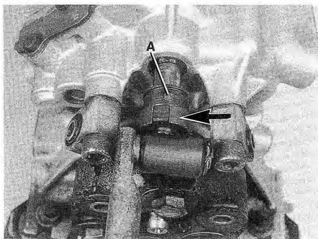
Fig. 4-5. Shift rod bushing lockring (arrow), and pin (A). Transmission shown removed. With transmission installed, drive pin out from below.
