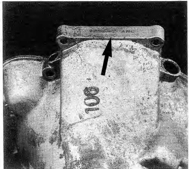
Fig. 1-4. Location of transmission identification code (arrow) on five-speed manual transmissions.
