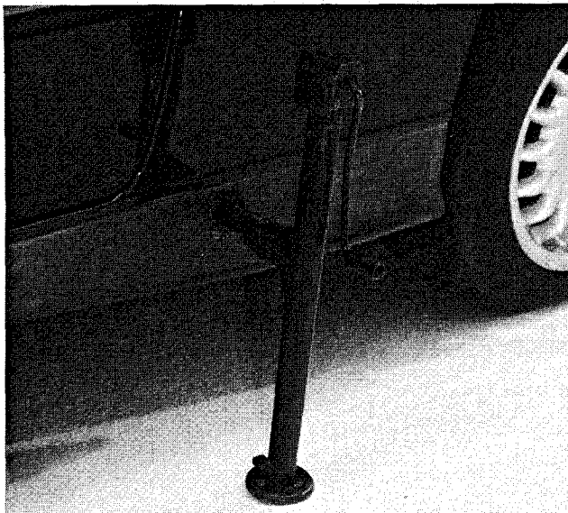
Fig. 3. BMW supplied jack correctly positioned in front jacking point.
