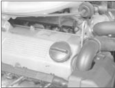
4.6a The threaded oil filler cap is located in the valve cover - always make sure the area around the opening is clean before unscrewing the cap
