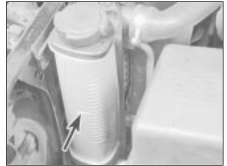
4.9a On some models, the expansion tank (coolant reservoir) is mounted on the radiator - make sure the level is kept at or near the FULL mark (arrowed)
