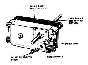
In the event of it being established that the gearboxes themselves are unduly noisy, apply to this Service Station for replacements and return the old gearboxes for examination.
