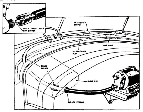
The windscreen wipers are operated by gearboxes and flexible cable drives from an electric motor mounted on the off-side front of the dash.
