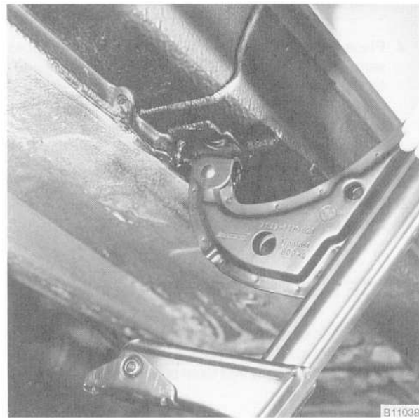
Fig. 2. BMW supplied jack correctly positioned under front jacking point.
