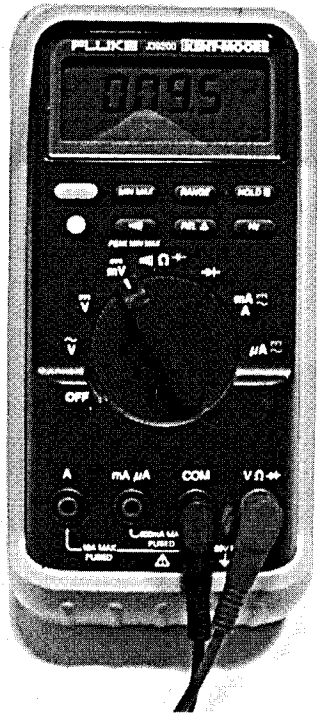
Fig. 16. Multimeter or Digital Volt/Ohmmeter (DVOM).
