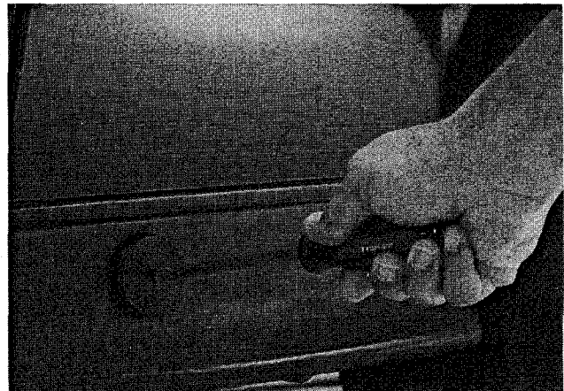
Fig. 2. Jack mount cover being removed from rocker panel.
