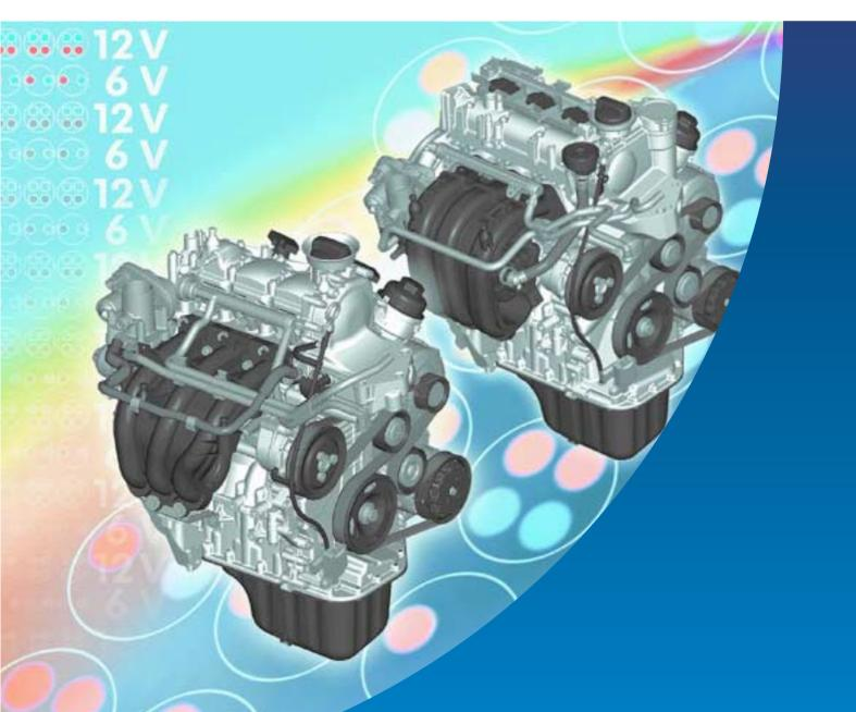
The two 1.2 ltr. engines mark the introduction of 3-cylinder petrol engines at Volkswagen. This pair of entry-level engines rounds off the range of engines of the 2002 Polo.
