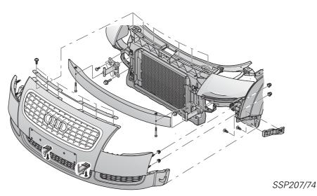
The front bumper comprises two parts: the cover panel and a decorative grille. The bumper carrier is made of aluminium and bolted to the side members by impact absorbing elements.
