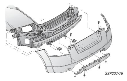
The rear bumper comprises a total of 4 parts: the bumper panel, the rear cover, the aluminium cross-member and the central locating element.
