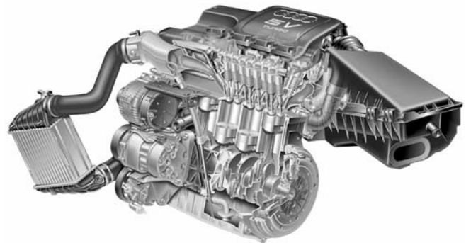
Turbo-charged and intercooled TT engine with 5 valves per cylinder as installed from the 2000 model year.
