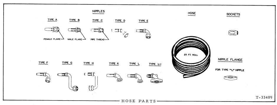
Refer to right hand column for identity of interchangeable crimped-type hose (fittings not re-usable). Assembly number shown in left hand column indicates available replacement hose assembly with re-usable components; where no assembly number is listed, hose assembly is not available from factory but may be constructed in the field from data indicated.
