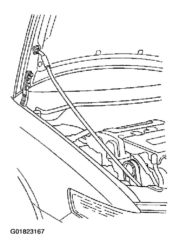
Fig. 1: Secure The Hood With Support Rod In The Lower Hole
