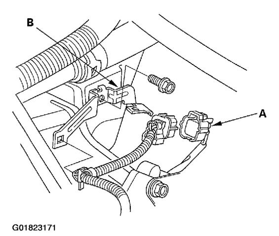
Fig. 5: Disconnecting The Secondary Heated Oxygen Sensor
