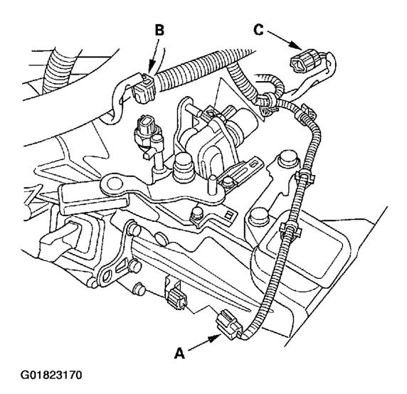
Fig. 4: Disconnecting The Countershaft Speed Sensor, Back-Up Light Switch, And Reverse **Lockout Solenoid Connectors**
