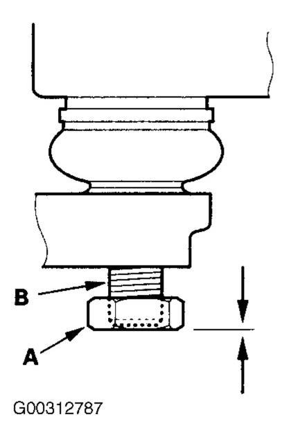
Fig. 3: Installing Hex Nut Courtesy of AMERICAN HONDA MOTOR CO., INC.
