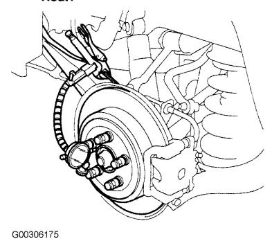
Fig. 2: Identifying Wheel Bearing End Play Courtesy of AMERICAN HONDA MOTOR CO., INC.
