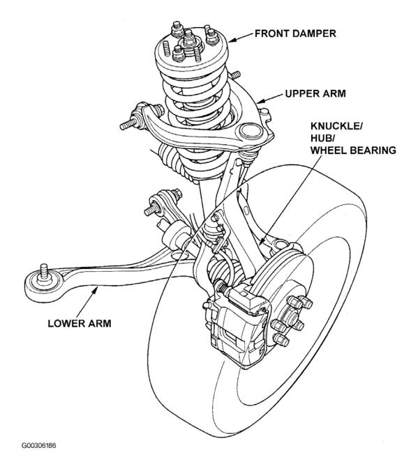
Fig. 1: Identifying Front Suspension Components
