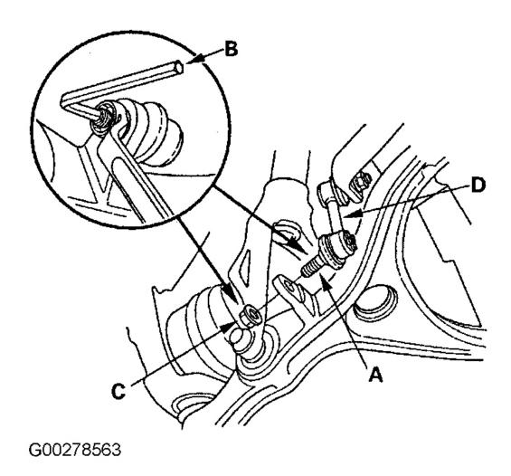
Fig. 3: Holding Stabilizer Ball Joint Pin With Hex Wrench **Courtesy of AMERICAN HONDA MOTOR CO., INC.**
