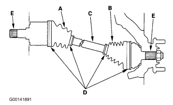
Fig. 1: Inspecting Boot & Boot Bands Courtesy of ISUZU MOTOR CO.
