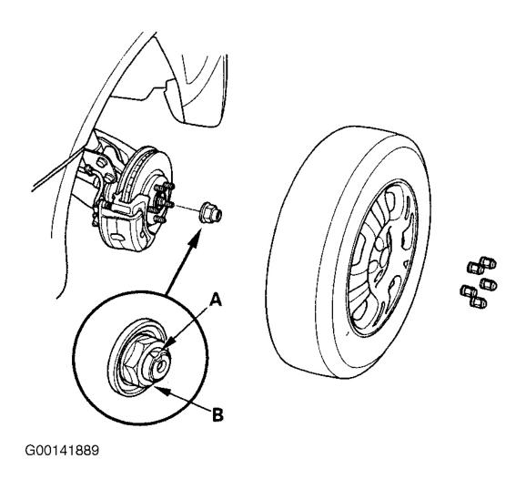
Fig. 2: Removing & Installing Axle Nut **Courtesy of AMERICAN HONDA CO., INC.**
