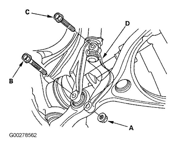
Fig. 4: Removing Self-Locking Nut & Flange Bolts Courtesy of AMERICAN HONDA MOTOR CO., INC.
