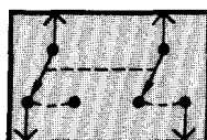
SWITCHES THAT MOVE TOGETHER DASHED LINE SHOWS A MECHANICAL CONNECTION BETWEEN SWITCHES
