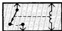
RELAY SHOWN WITH NO CURRENT FLOWING THROUGH COIL WHEN COIL IS ENERGIZED, SWITCH IS PULLED CLOSED
